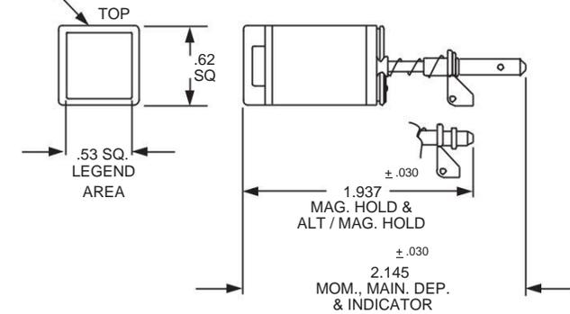
Typical of B, C and D pushbutton styles.
