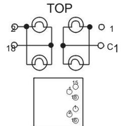
Lamp schematic only. For switch and coil terminal numbers and positions refer to standard magnetic holding diagrams above.
