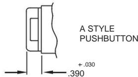
Tolerances: Unless otherwise specified - Fraction  $\pm 1/32"$ , Note: Only standard and "A" style pushbuttons may be used with Type II.
